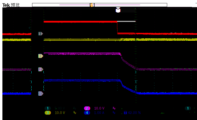
Figure 24. IN Off resistive load 1A
